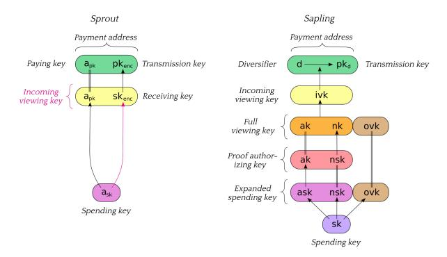
[Sprout] The receiving key  $sk_{enc}$ , the incoming viewing key  $ivk = (a_{pk}, sk_{enc})$ , and the shielded payment address  $addr_{pk} = (a_{pk}, pk_{enc})$  are derived from  $a_{sk}$ , as described in § 4.2.1 'Sprout Key Components' on p. 28.
